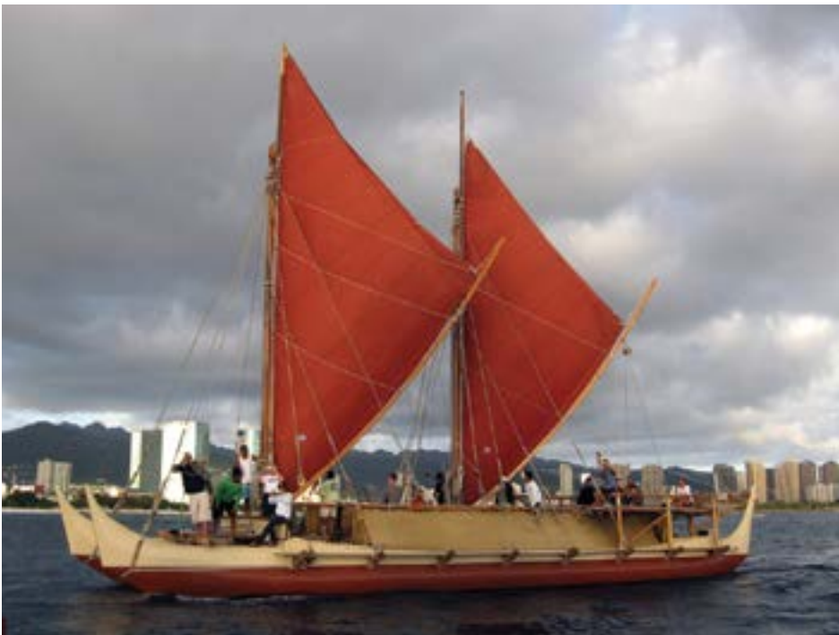
FIGURE 2-3 The Hokule'a . This vessel is a reproduction of the double-hulled voyaging canoes that the Polynesians used to explore and colonize the Pacific.
