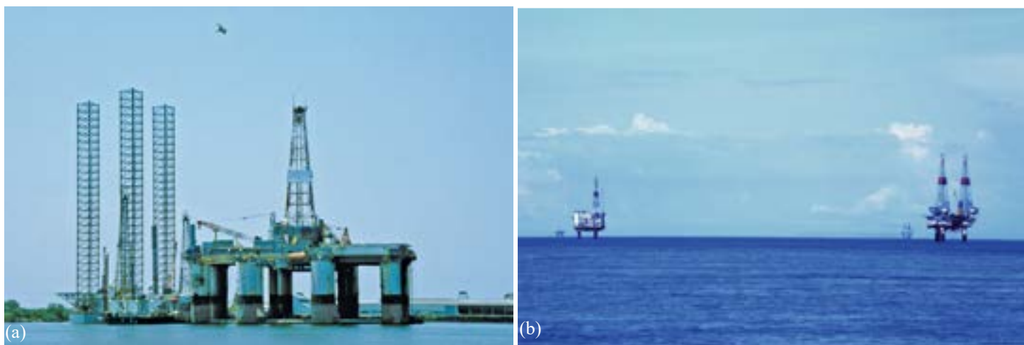
FIGURE 2-12 Structures of the offshore oil and gas industry. (a) These offshore exploration drilling rigs are under maintenance in Galveston, Texas. On the left, a typical jack-up drilling rig; on the right, a typical floating rig that rides on pontoons below the depth of most wave action. (b) Production oil rigs permanently emplaced in the seafloor of Cook Inlet, Alaska
