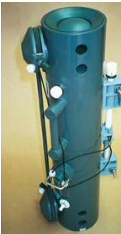
FIGURE 3-10 A GoFlo water-sampling bottle. This ingeniously designed bottle is lowered through the sea surface in a closed configuration to avoid contamination. At a depth of a few feet, a pressure-sensitive trigger opens both ends of the bottle. The bottle is closed again by means of a messenger or other triggering device when the bottle is at the required sampling depth.
