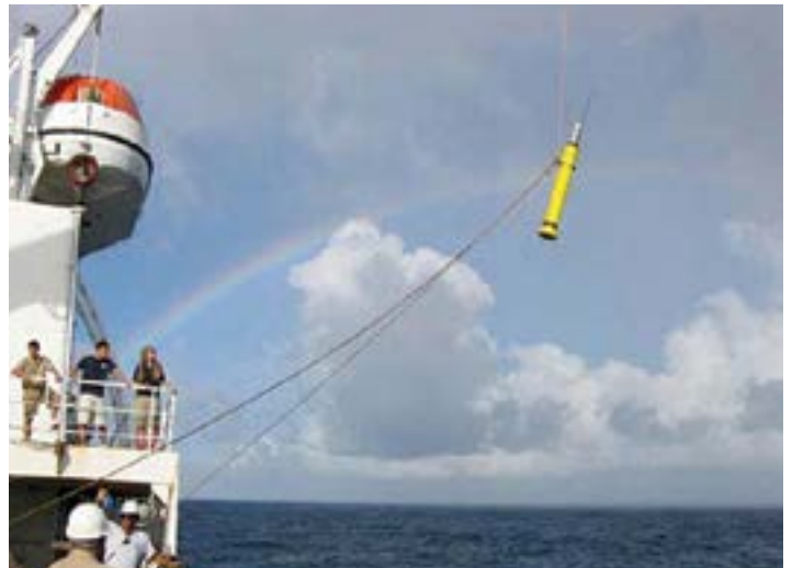
FIGURE 3-23 The yellow cylindrical object is an Argo float system about to be deployed from a research vessel to begin its long unattended journey through the ocean depths.
