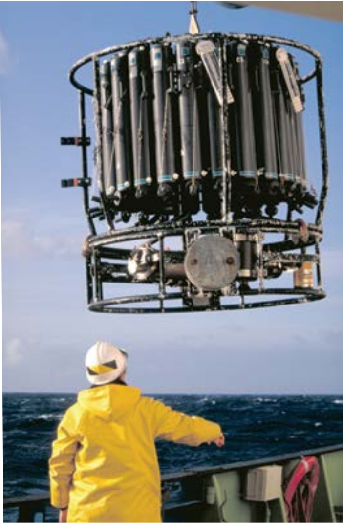
FIGURE 3-12 Rosette water sampler. The sample bottles, some fitted with thermometer racks, are arranged in a rosette pattern around an electronic device that enables researchers on the ship above to close individual sample bottles at selected depths through an electrical signal sent down the hydrographic cable. The round frame below the water-sampling bottle rack usually contains a CTD and possibly other sensors, such as turbidity-measuring devices.
