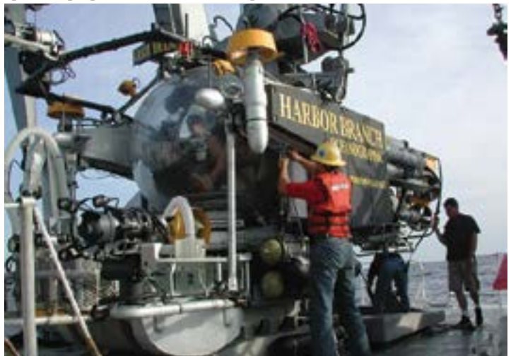
FIGURE 3-21 A typical submersible, such as the Johnson Sea Link shown in this photograph, consists of a glass or plastic sphere inside a hull. The scientists descend within the sphere, which is provided with air and heat. Motors, articulated arms, and many different designs of samplers and cameras are mounted outside the sphere. These are used to provide propulsion and collect samples
