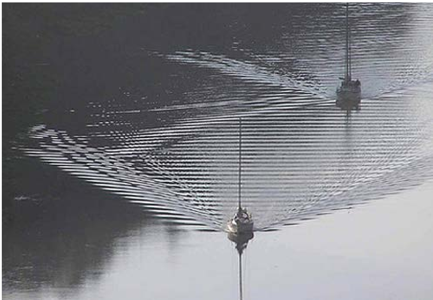
FIGURE 9-11 A boat's bow and stern waves travel out from the ship as wave trains. If you look carefully at the bow wave of the leading boat you can see that the leading wave disappears as it moves away from where the boat has passed and is replaced by another wave behind it. The second wave in turn also disappears, to be replaced by another one behind it, and so on. The wave energy is slowly spread as the wave crest lengthens by dispersion, and the wave train eventually disappears. Note how the bow and stern waves of the two boats combine to form complex wave interference patterns.
