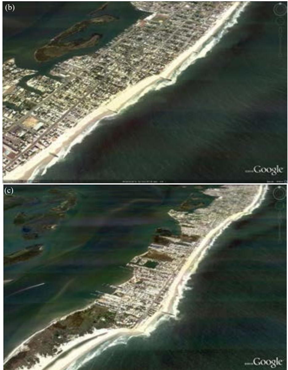
FIGURE 11-22 Groins designed to stop beach erosion modify the longshore sand transport and, consequently, the beach. (a) Sand accumulates on the upcurrent (longshore drift current) side of the groin and is eroded from the downcurrent side. (b) Often a line of groins is constructed along the length of a beach, which creates a saw-toothed beach shoreline like this one at Beach Haven, New Jersey. The groins will not provide effective protection as sea level rises and this barrier island recedes in the same way as Galveston island (Fig. 11-21). (c) You can see that the barrier island on which Beach Haven is built has already retreated in the undeveloped and unprotected area just south of the area shown in (b). Within perhaps 50 years, all the structures that you see on this barrier island will be gone or will require massive seawalls entirely around the perimeter of the island to protect them.
