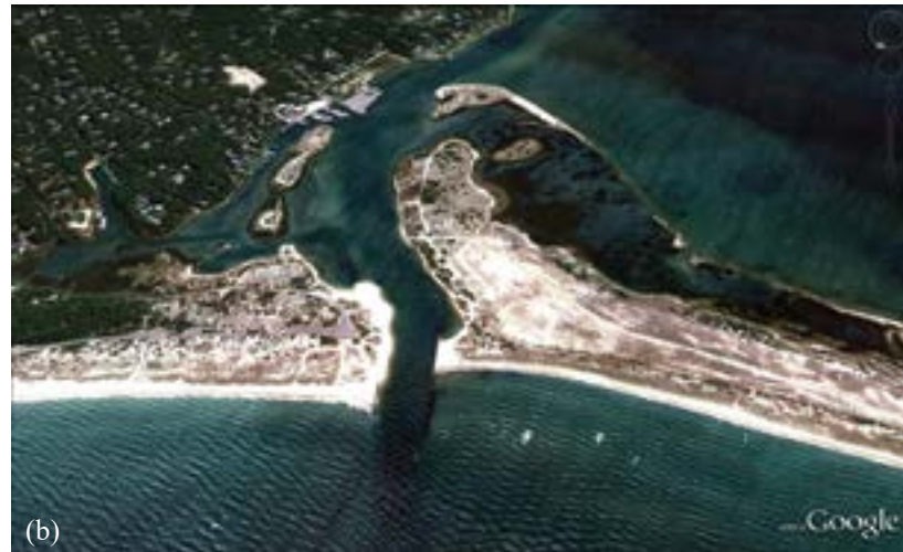
FIGURE 11-23 (Above) Jetties. (a) Rock jetties are often constructed on either side of an inlet between barrier islands to prevent silting of navigation channels and erosion of the sides of the inlet by waves from boats' wakes. These jetties obstruct the longshore sand transport, leading to the accumulation of sand and widening of the beach on the upcurrent side, and erosion and loss of the beach on the downstream side. (b) Three Mile Harbor, East Hampton, Long Island, New York. Can you tell which direction the longshore drift is?
