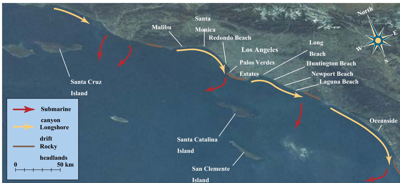
FIGURE 11-16 There are several north-to-south littoral drift cells in southern California. Each of these cells ends at the head of a submarine canyon where the sand is lost as it is transported down the canyon.
