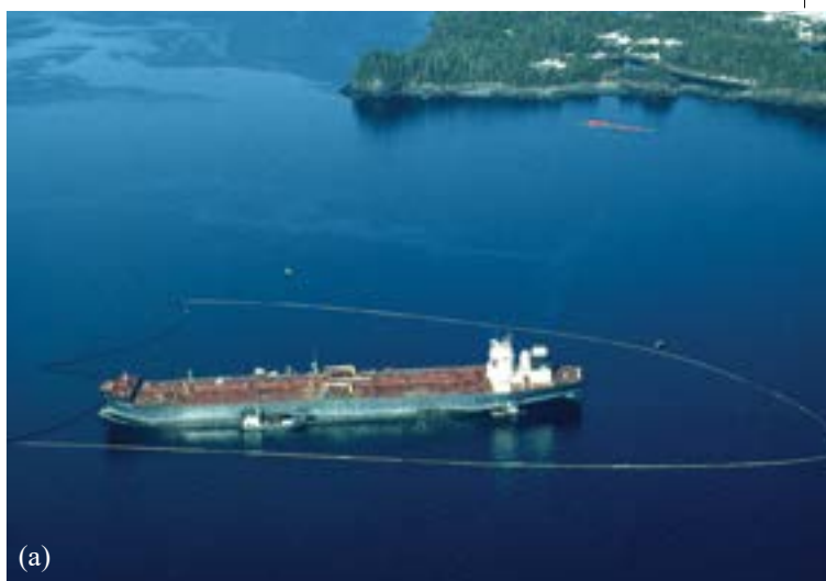
FIGURE 16-4 Oil spills provide spectacular images that ensure media coverage. (a) The Exxon Valdez tanker 48 h after it ran aground on Bligh Reef in Prince William Sound, Alaska, in 1989. In this photograph, the tanker is seen still leaking some oil, and it is surrounded by a boom that has been placed on the water surface in an attempt to contain this oil so that it can be collected. (b) A rescuer tries to capture an oiled Pelican after the 2010 Deepwater Horizon spill in the Gulf of Mexico. Rarely do heavily oiled birds survive even when cleaned up.
